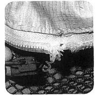
Fig. 40. Zipper Teeth Broken
